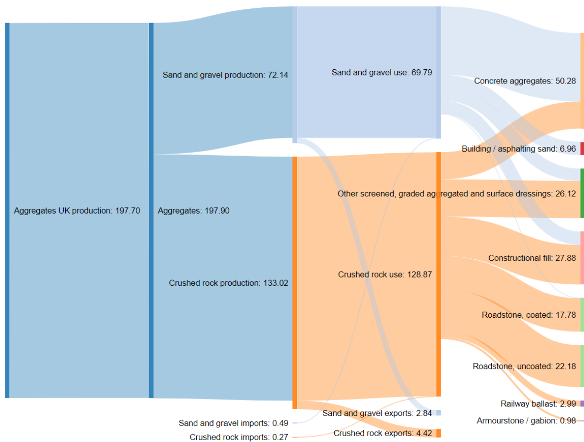
Figure 5-1 Production of aggregates (in Mt) in the UK, and potential end-use pathways. The gaps in the end use pathways may be due to: 1) use of data from Great Britain only; 2) data sets used are from different years; 3) discrepancies in the data sets used.
