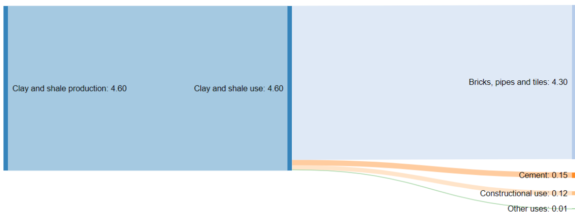
Figure 5-2 A cradle-to-gate mass flow depiction of clay and shale production and potential application pathways (in Mt) in the UK in year 2018.
