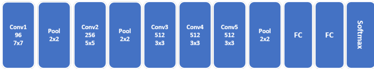
Figure 3.6: A 2D linear CNN with five convolutions and two fully connected layers
