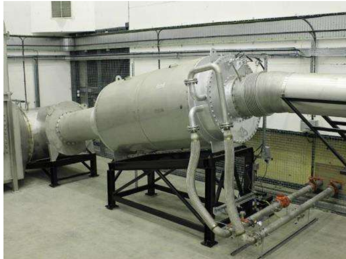
Figure 19: Photograph of an exhaust-to-thermal oil HPHE tied to an ORC cycle [98].
