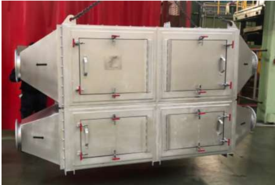
Figure 61: Experiment 3 photograph of HPHE during installation.
