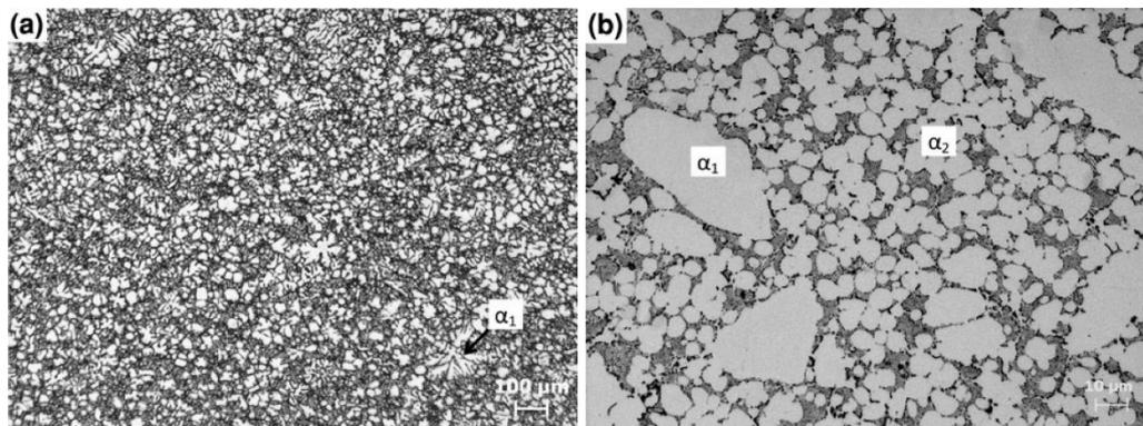
Figure 2. Microstructures of diecast Al-5Mg<sub>2</sub>Si-2Mg with 0.6Mn-0.2Ti alloy, (a) low magnification image showing the distribution of the primary  $\alpha_1$ -Al phase, and (b) high magnification image showing details of the morphology of the primary  $\alpha_2$ -Al phase solidified within the die cavity.
