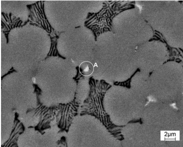
Figure 3. Backscattered SEM micrograph showing the eutectic and intermetallics of diecast Al-5Mg<sub>2</sub>Si-2Mg with 0.6Mn-0.2Ti alloy.
