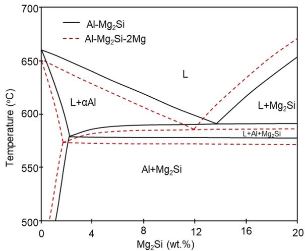
Figure 1. Equilibrium phase diagram of pseudo-binary Al-Mg<sub>2</sub>Si and Al-Mg<sub>2</sub>Si-Mg system.
