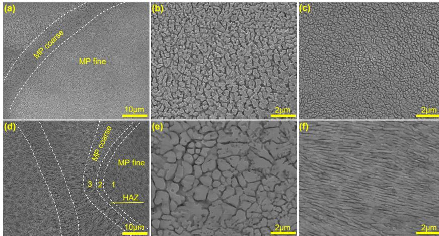
Figure 5. SEM images showing (a) the overall microstructure, (b) the detailed microstructure in zone 3, and (c) the detailed microstructure in zone 1 along the horizontal direction; (d) the overall microstructure, (e) the detailed microstructure in zone 3, and (f) the detailed microstructure in zone 1 along the building direction in the SLM fabricated Al-5Mg<sub>2</sub>Si-2Mg alloy. 1- MP fine zone, 2- HAZ (heat affected zone), 3- MP coarse zone.
