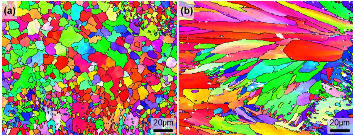
Figure 4. EBSD images of as-SLM Al-5Mg<sub>2</sub>Si-2Mg alloy along (a) the horizontal direction (in cross section parallel to base plate), (b) the building direction (in cross section perpendicular to base plate), and (c) corresponding IPF map.
