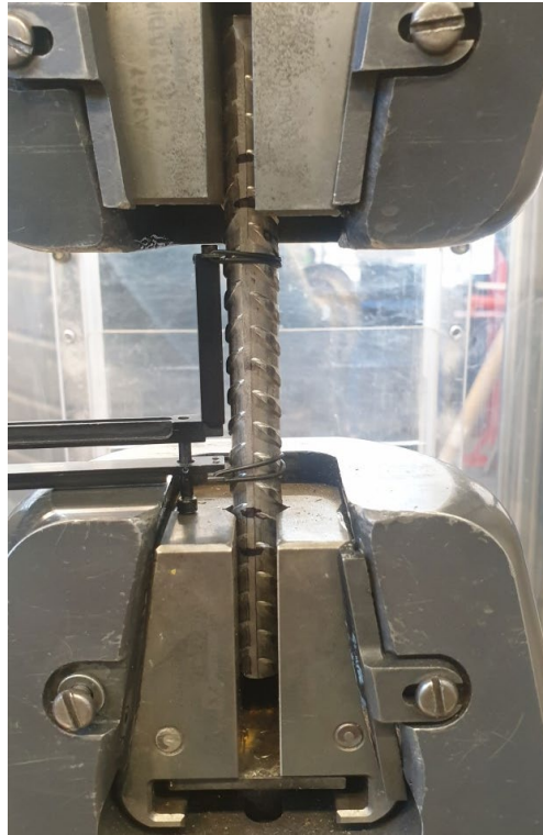
Figure 4 – Complete tensile testing setup on the Instron 5584, with the Instron EX2620-601 extensometer.
