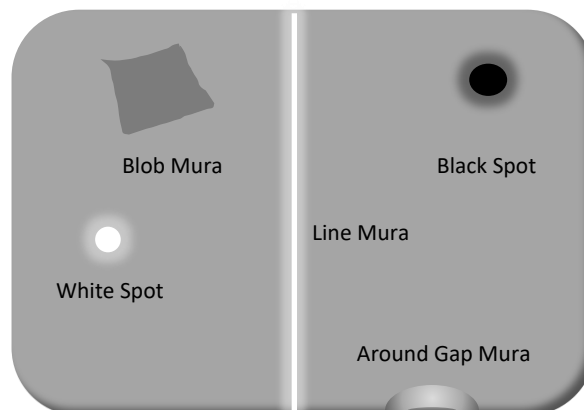
Figure 2.5: Mura defect types
