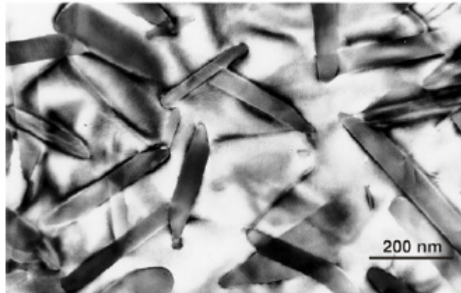
Figure 2.8- \beta -phase precipitates in AZ91 sample aged for 8 hours at 200°C (Nie, 2002)
