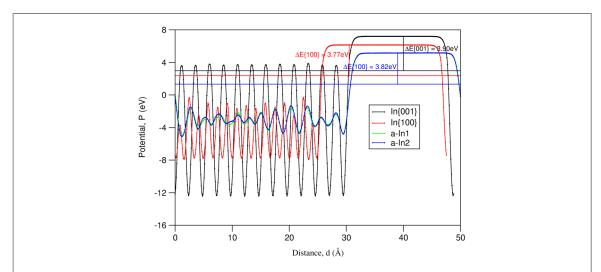
**Figure 8.** Planar averages of the local potentials, related Fermi levels (horizontal lines) and work functions obtained with equation (2) for In {001}, In {001} and two a-In samples.
