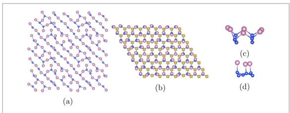
Figure 3. The atomic arrangements and interfacial Si-In bonding for (a, c) the Si $\{0\ 0\ 1\}$ -In and for (b, d) the Si $\{1\ 1\ 1\}$  interfaces, respectively. The blue and violet spheres represent interfacial Si and In, while the yellow-crossed blue spheres represent Si at the subsurface layer. The cut-off Si-In bond-length is 3.15 Å.
