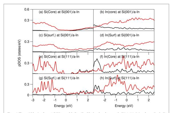
$\textbf{Figure 5.} \ \ The partial density of states (pDOS) around the Fermi level for the selected atoms at the Si \{0 0 1\}/a-In interfaces and at the Si \{1 1 1\}/a-In interfaces. The labels (core) or (surf.) indicate the atom at the core of the slab or the surficial atom, respectively. The Black and red curves represent the s-characters and the p-characters, respectively. The Fermi level is at 0 eV.$
