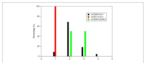
$\textbf{Figure 4.} \ \ \text{Distribution of the number of closest nearest neighboring Si atoms for the interfacing In atoms at the simulated c-Si/a-In and c-Si/c-In interfaces.}$
