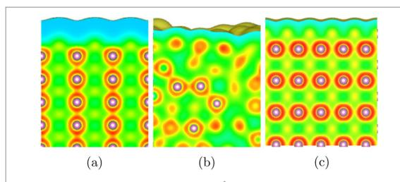
**Figure 7.** Electron density distribution with iso-surfaces  $(1.0 \times 10^{-5} \text{ e/Å}^3 \text{ at the outer skin of the slab)}$  for (a) c-In{1 0 0}, (b) a-In, and (c) In{0 0 1} surfaces. The silvery spheres represent In atoms. The electron density decreases from red to yellow, to green to sky-blue and ends at dark yellow (iso-surfaces).
