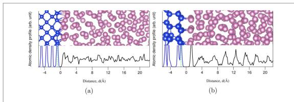
Figure 2. Snapshot (top) and related atomic density profile (bottom) for (a)  $Si\{0\ 0\ 1\}/a$ -In and for (b)  $Si\{1\ 1\ 1\}/a$ -In. The blue spheres represent Si and violet In. The cut-off Si-In interatomic distance is  $3.15\ \text{Å}$ .
