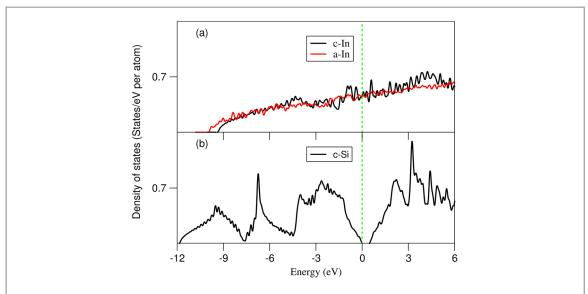
Figure 1. Density of states (DOS) for elemental (a) In and (b) Si. The Fermi level (In) and top of the valence band (Si) is at 0 eV (the green line).
