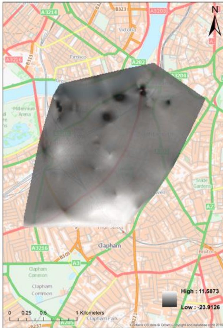
Figure 5. 11 – Maps showing the level of London Clay (left) and Lambeth Group (right) across the mapped Battersea to Nine Elms area derived from borehole data.
