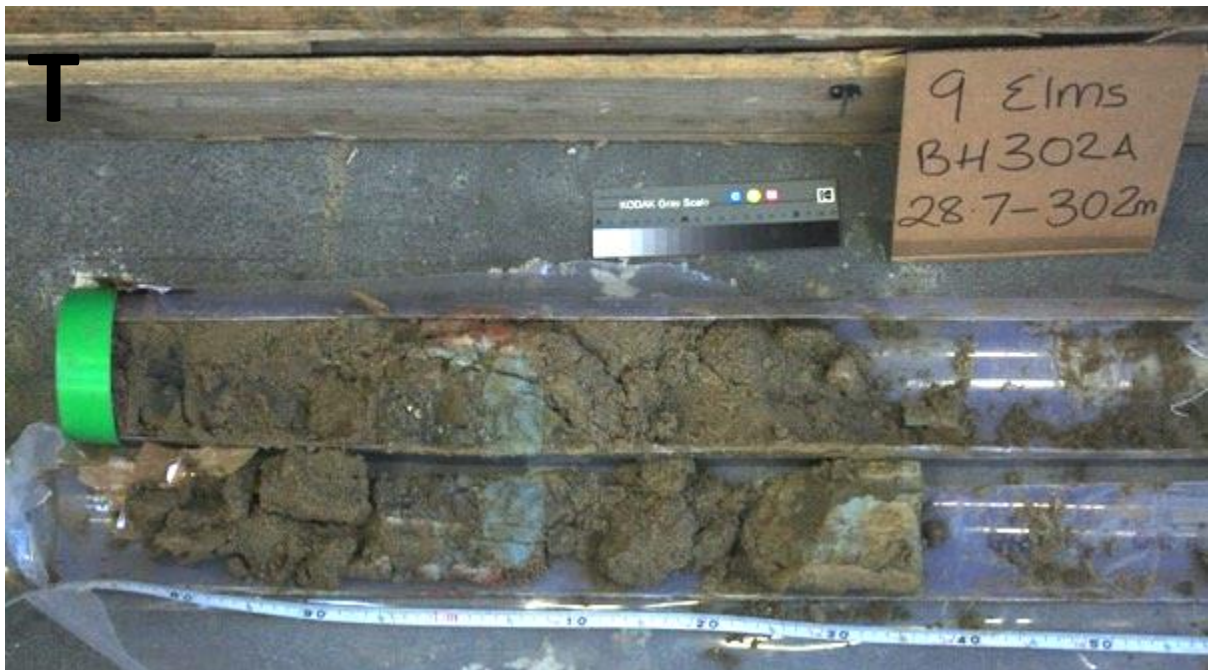
Figure 5. 38 – Borehole 302a from One Nine Elms at 28.7-30.2 m deep. Intact sections of mottled beds from the Lambeth Group within sand and gravel sediment. "T" shown to identify the direction of the top of the borehole.
