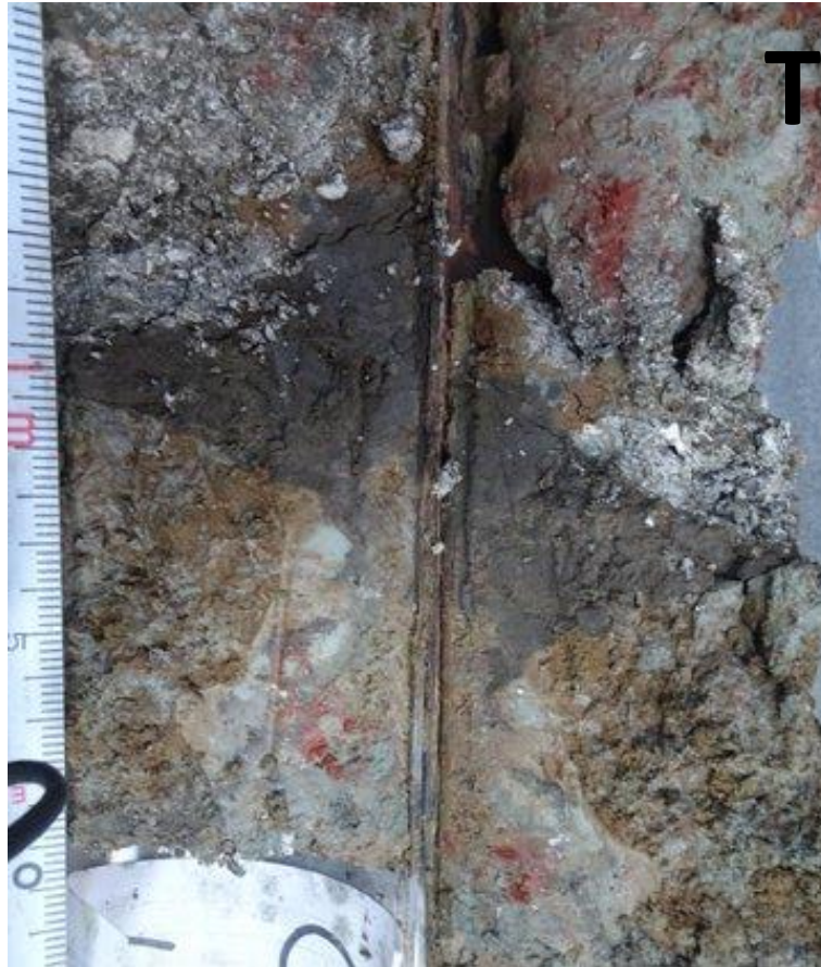
Figure 5. 37 - One Nine Elms at 41 m deep. Calcification, Lambeth Group and a dark grey layer (potentially the mid-Lambeth hiatus) unusually banded. "T" shown to identify the direction of the top of the borehole.
