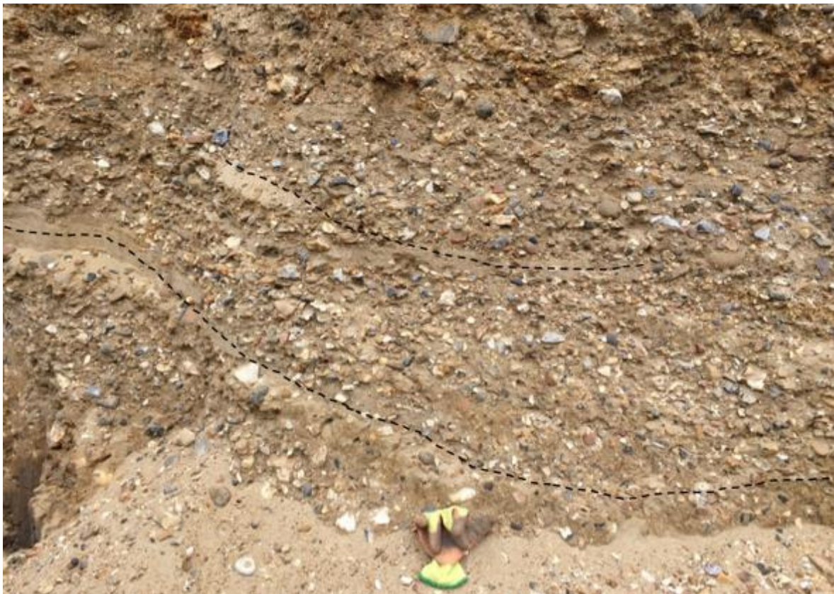
Figure 5. 30 – Infill material at Battersea Power Station Phase 3. The infilling material shows two distinct sand layers where gravel is not present. The sand layers are dipping towards the centre of the feature. Exposure is approximately 2.5 m wide and 2 m high.
