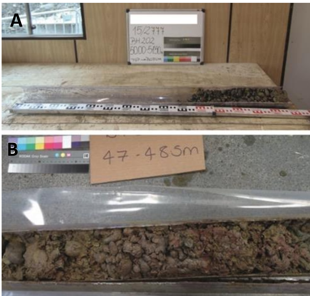
Figure 4.3 - Images depicting gravel retrieval via a rotary drill rig. Image A shows a lack of retrieval of the unconsolidated gravel sediment. Image B shows the retrieval of gravel sediment when there are finer particles present to consolidate the larger gravel sediment.
