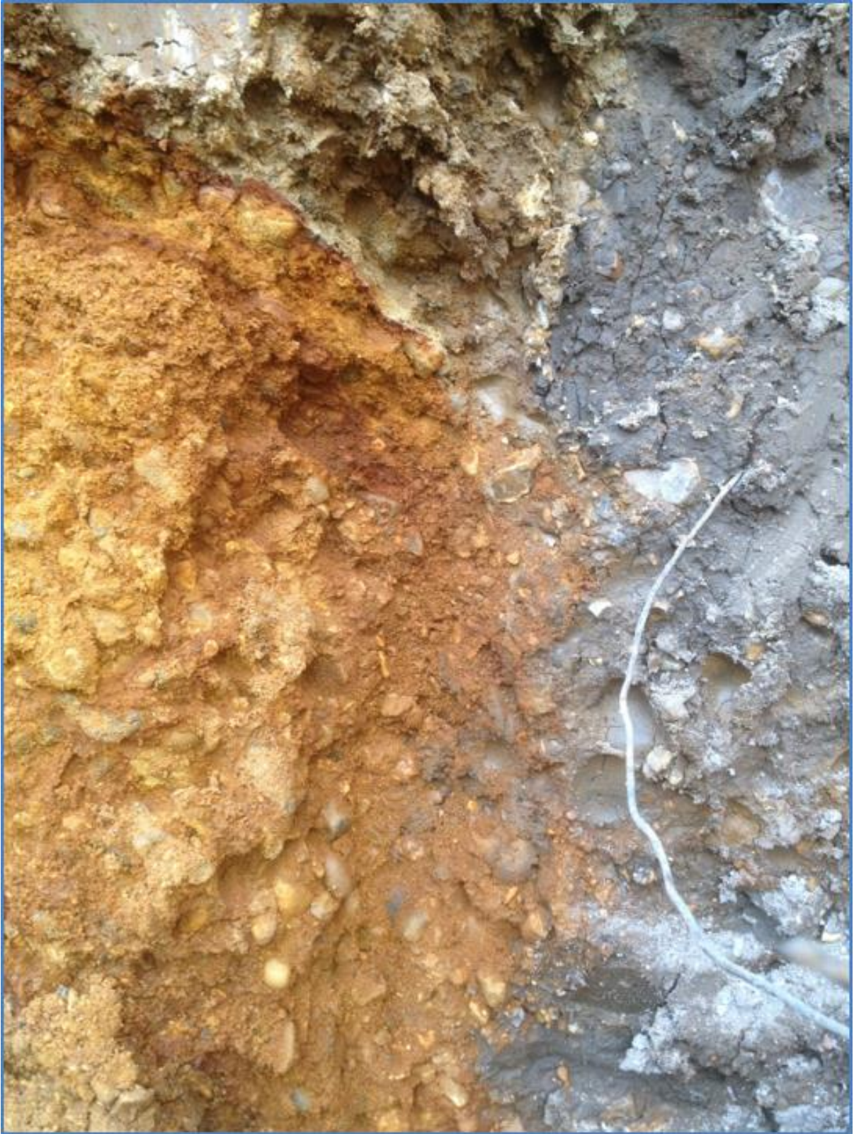
Figure 9.10 – DFH infill showing the contact between silt, clay and RTDs.
