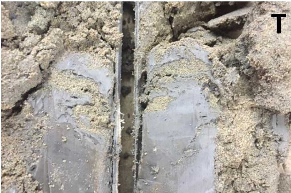
Figure 5. 36 – Borehole 303 from One Nine Elms at 21.5 m deep. Horizontal sand intrusions in the London Clay. “T” shown to identify the direction of the top of the split borehole.
