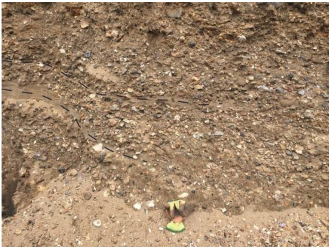
Figure 4.5 - The dipping sand layers, indicated by dashed lines, would not have been able to be interpreted from a borehole. This larger exposure aids scientific research to understand previous processes associated with the feature and its infill which otherwise would not have been possible. Exposure is approximately 2.5 m wide and 2 m high.
