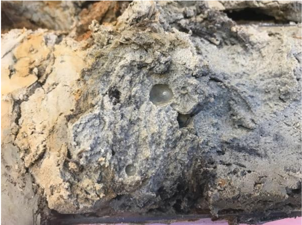
Figure 5. 34 – Bubble-like structures identified within the fine sand, silty, clayey material at Ashford Hill. The largest bubble shown in the centre of the image is around 0.8 mm.
