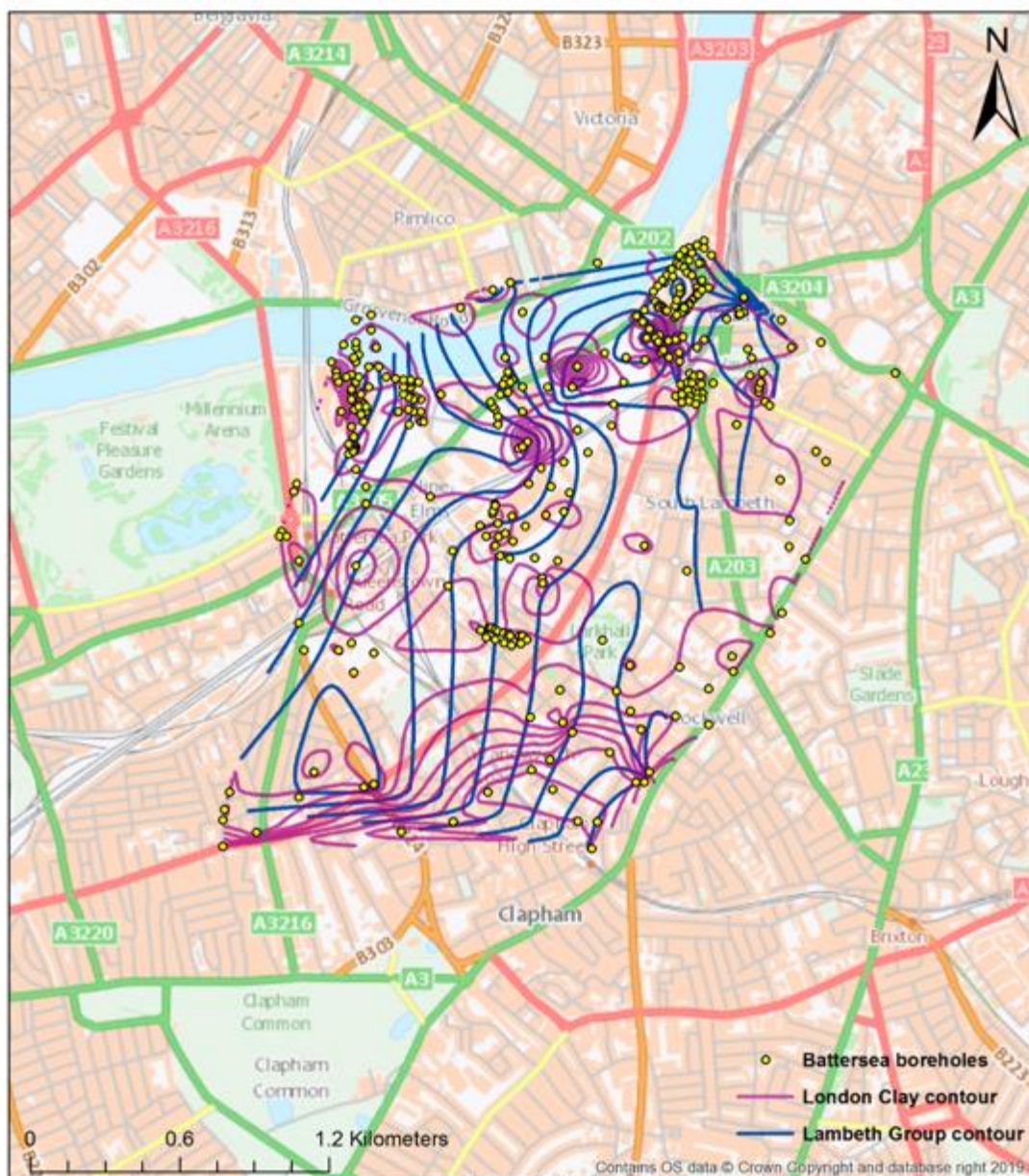
Figure 3. 21 - The contour results for the top of the units for the Battersea mapped area including the boreholes used for the analysis.
