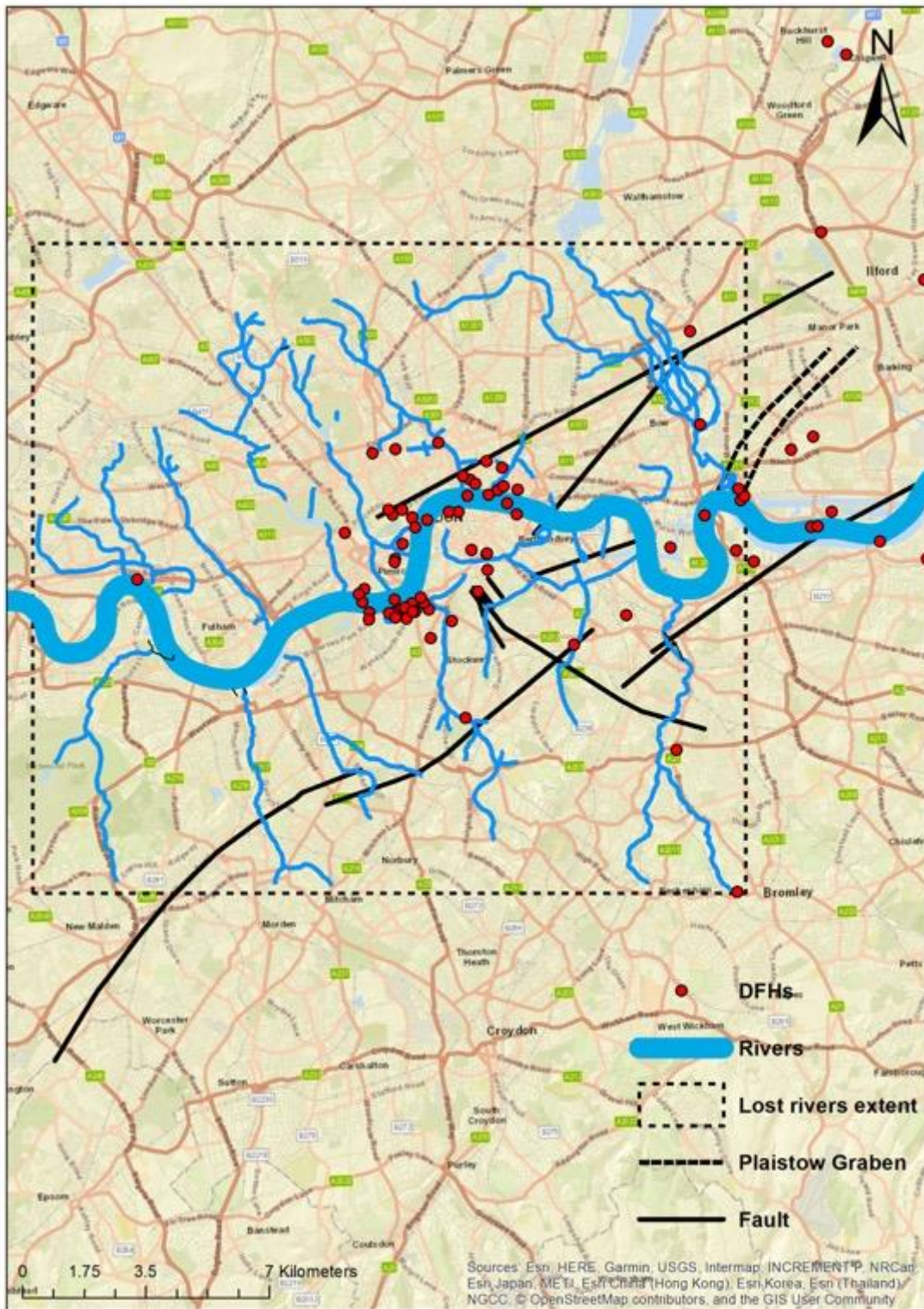
Figure 5.9 – Location of DFHs in relation to major known faults and the rivers (including lost, taken from Barton, 1992) of London. The known limits of the lost rivers of London are shown within the dashed box.
