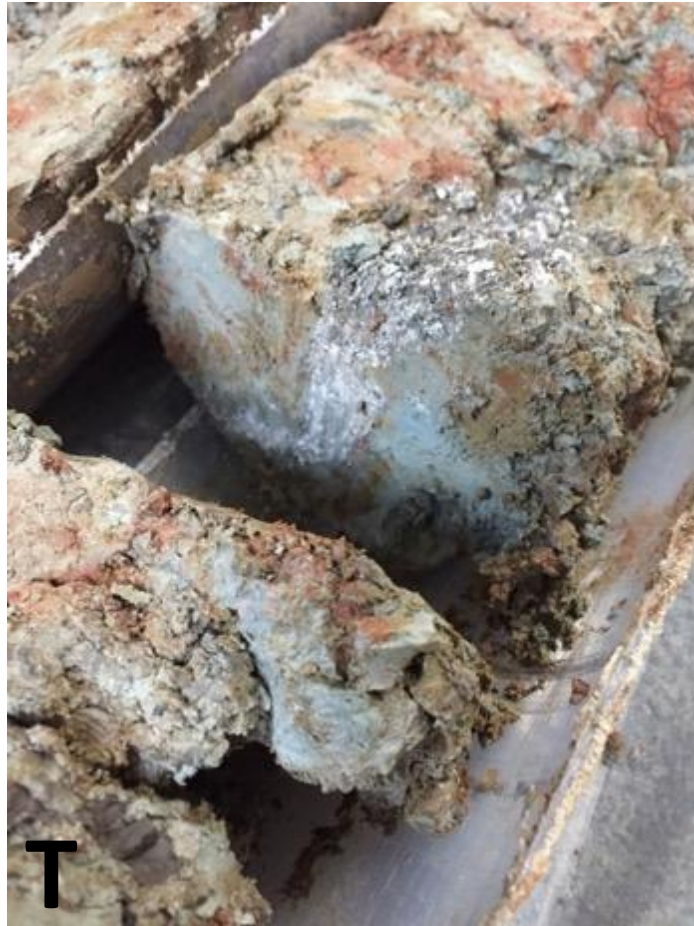
Figure 5. 35 – Borehole 302a from One Nine Elms at 30.4 m deep. Displaying a calcrete vertically embedded within the Lambeth group. “T” shown to identify the direction of the top of the borehole.
