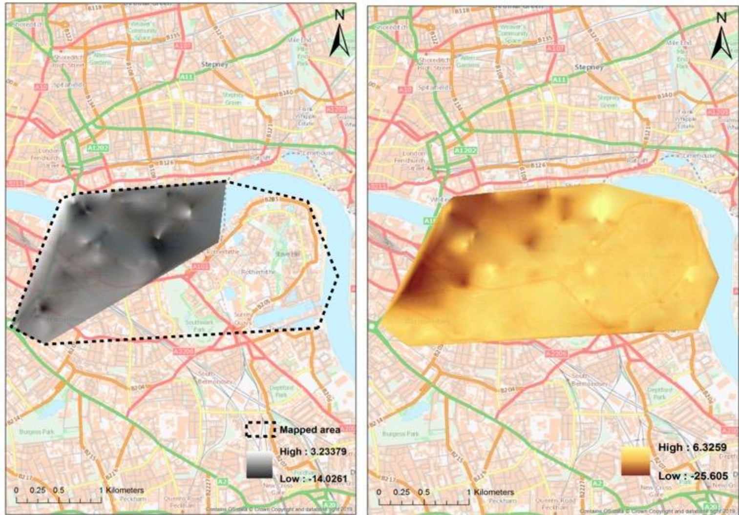
Figure 5. 12 - Maps showing the level of London Clay (left) and Lambeth Group (right) across the mapped Bermondsey area derived from borehole data.
