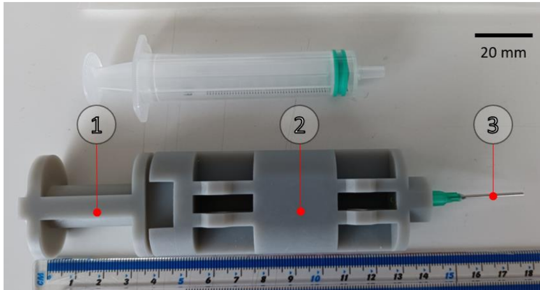
Figure 6.6 – Sample Collection Device fabricated using SLA printing (2 nd iteration) 1, Swab Receiver; 2, Redesigned Lower Section containing both switch valves; 3, Dispenser Tip Needle
