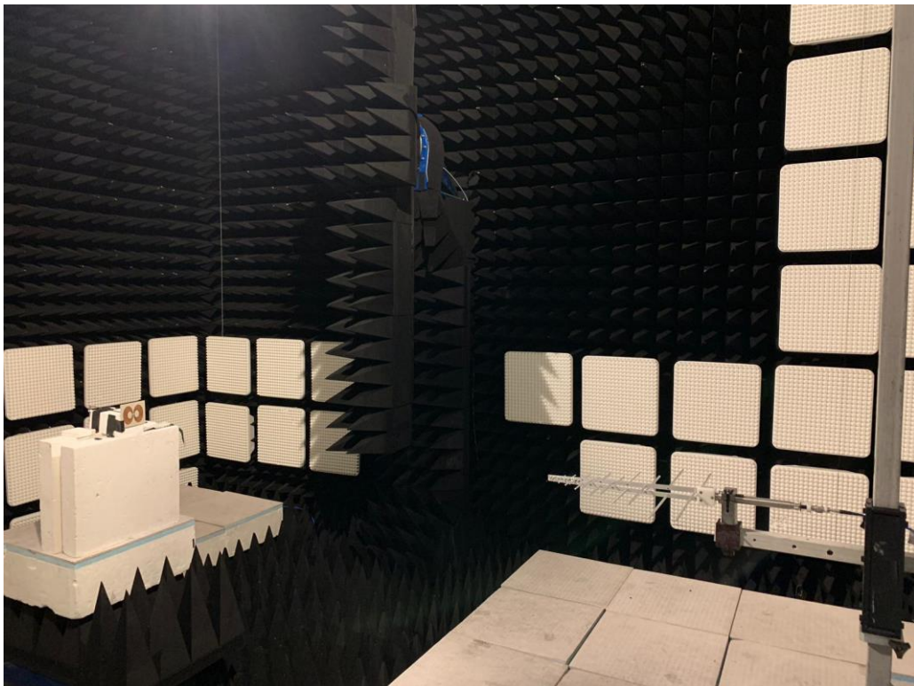
Figure 35. Measurement of planar elliptical dipole antenna in an anechoic chamber at NPL, UK 2
