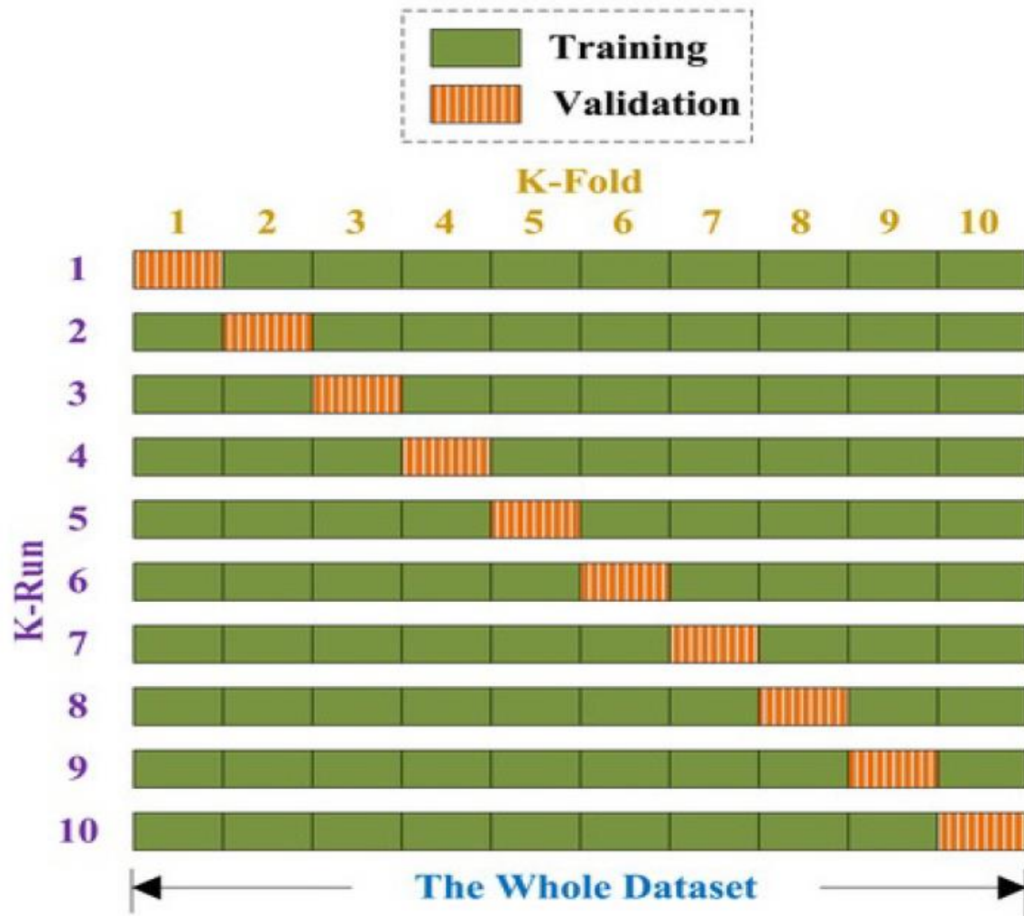
Figure 3.7: Diagram of a 10-Fold Cross Validation (Bosoni, 2016)
