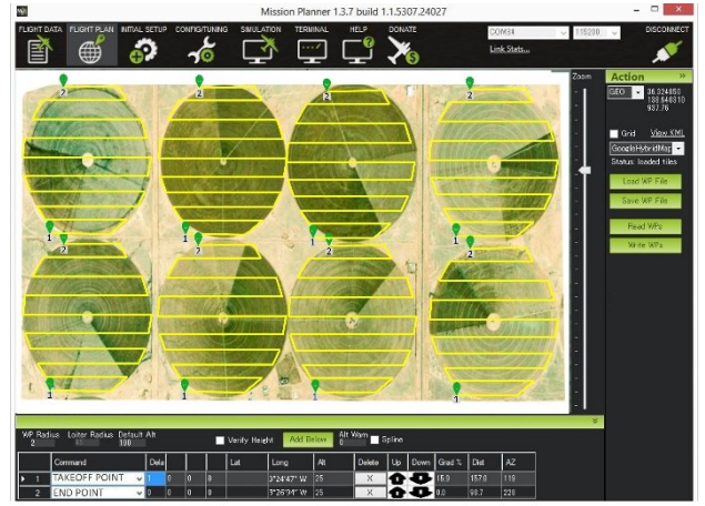
Fig. 4: Crop monitoring using a Mission Planner tool
