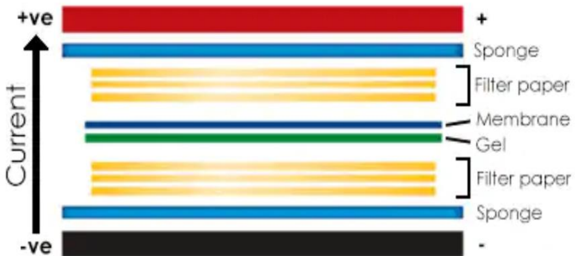
Figure 7.3: Order of assembly for the protein transfer 'sandwich' . Once the SDS polyacrylamide gel containing protein samples was run, the protein transfer 'sandwich' to transfer the proteins onto a nitrocellulose membrane was prepared as shown above. The sponges, filter papers and nitrocellulose membrane were pre-soaked in 1X transfer buffer prior to assembly. Image from: abcam.
