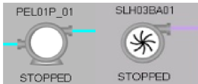
Figure 4-9 Example of new pump and blower symbols [97]
