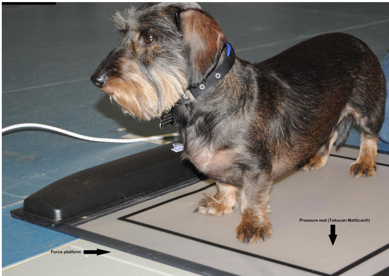
Fig. 1 One of the dogs in quiet standing during a measurement on a synchronised pressure mat (Tekscan Matscan®) on top of a force platform
