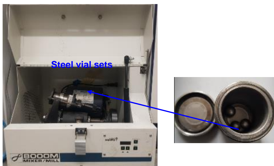
Figure 4. 7: Ball Milling: Spex Certi-Prep 8000M mixer set, reactor vessel with Hardened Steel Vial Sets milling balls of 11mm diameter
