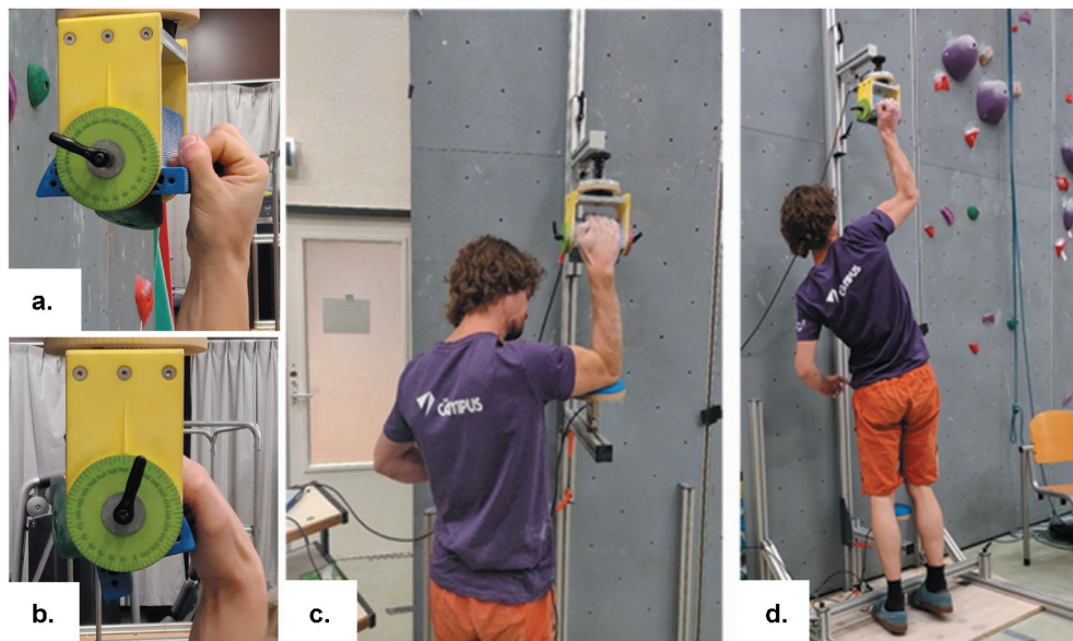
Figure 1. Assessing peak force producing capabilities using different grip types, i.e. at the fingertips using an edge (a) and hand using a slope (b), and using different positions, i.e. either elbow isolated (c) or free, open chain (d) positions. Note the bar at the feet in (d) which was useful for participants who were able to pull more than their body mass.
