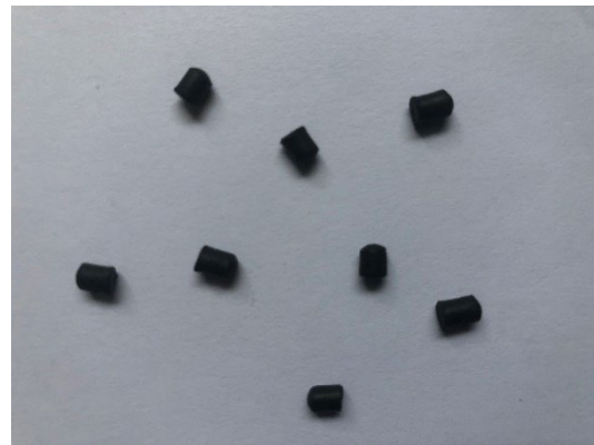
Fig. 2. Recycled PVC plastic aggregates
