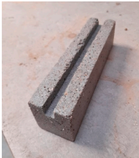
Fig. 3. Concrete prisms to be retrofitted.
