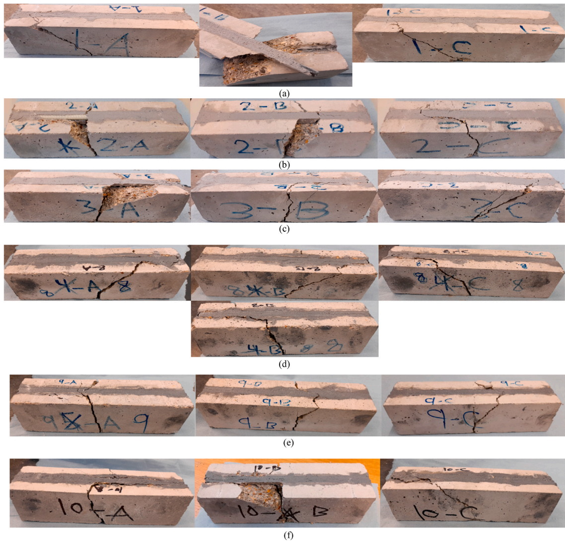
Fig. 7. Failure modes of specimens (a) C-NE-8, (b) G-NE-8, (c) B-NE-8, (d) C-Gr-0.1-8, (e) G-Gr-0.1-8 and (f) B-Gr-0.1-8.
