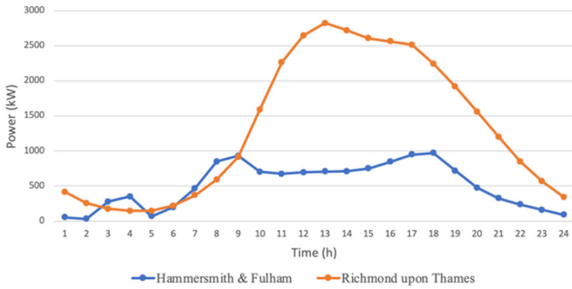
Fig. 3: Case studies in two London boroughs for SHBS charging stations Table 1 displays the primary technical and economic parameters of each station. For the case study, a 24-hour scheduling period was employed, with an hourly energy dispatch solution used on a summer reference day. The common parameters of the charging stations include:
