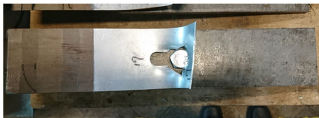
Specimen 2.0-10-wo-75 Bearing failure
