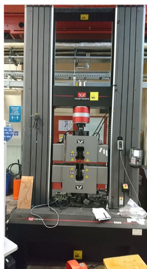
Universal Testing Machine for shear connection test
