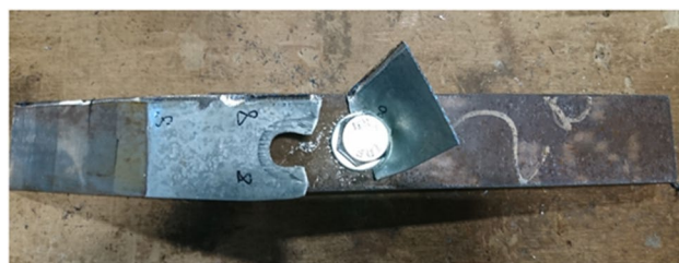
Specimen 1.2-15-w-50 Net section failure
