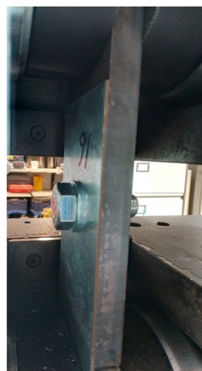
Specimen fixed by the mechanical grips
