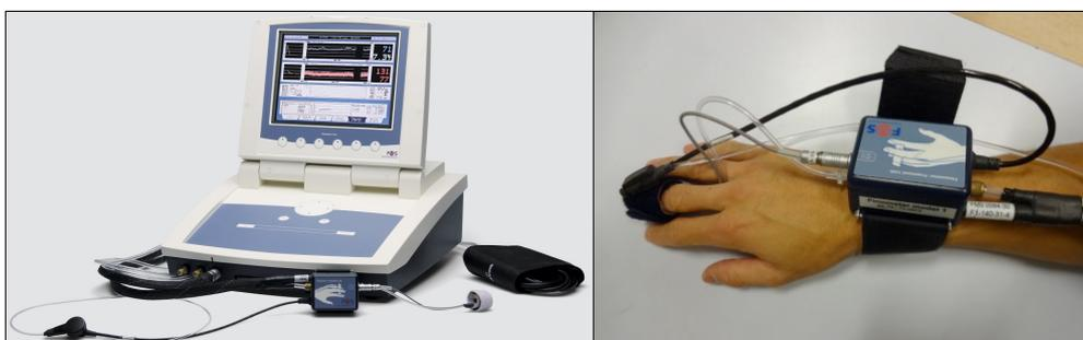
**Figure 14. Finometer equipment.** Image on the left illustrates the Finometer infrared photoplethysmography device (reproduced from Finapres.com, FMS, Netherlands). Image on the right demonstrates the fitting of the device on the participant's wrist and middle finger.
