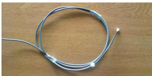
**Figure 12. Image of rectal temperature probe.** The probe (Ret-1 Special, Physitemp, Clifton, NJ, USA) was self-inserted 15 cm past the sphincter muscle.
