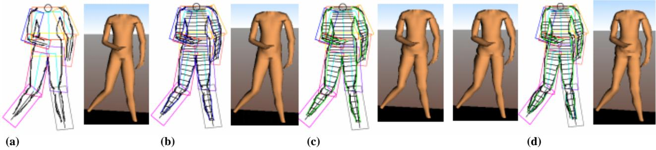
**Figure 3. (a) The input 2D freehand sketch and the 3D model after rigid morphing. (b) Graphical comparison to get the fat distribution measurements and the fatness morphed model (c) Graphical comparison to get the surface fitting measurements; the model with and without system auto-beautification (d) Overtracing body contour (right lower torso, and lower legs) to modify an existing 3D surface model.**
