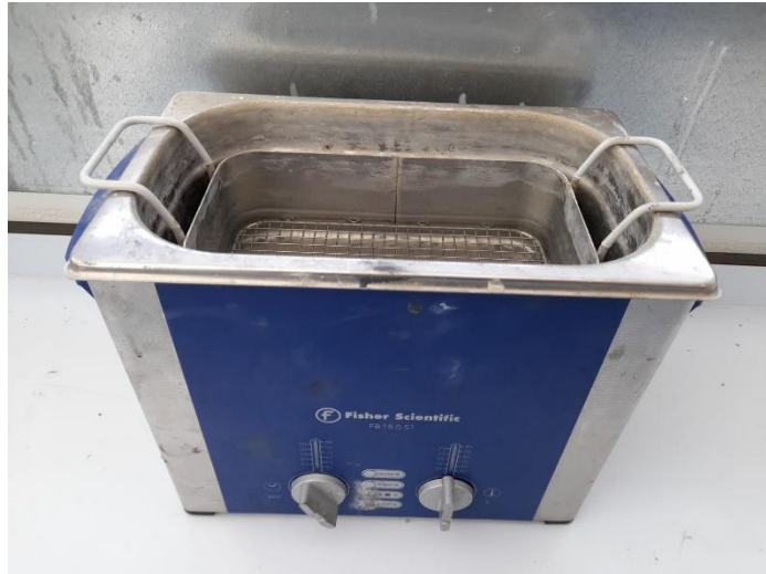
Fig. 3.5 The Fisher Scientific FB 15051 ultrasonic bath.
