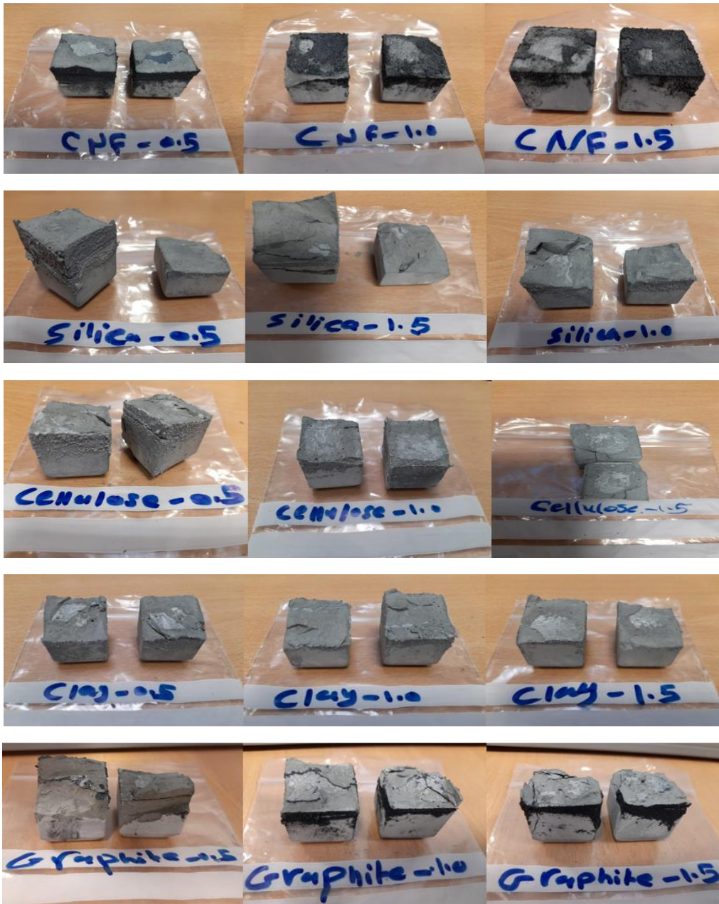
Fig. 5.1 Failure modes of the CP-adhesive joints.
