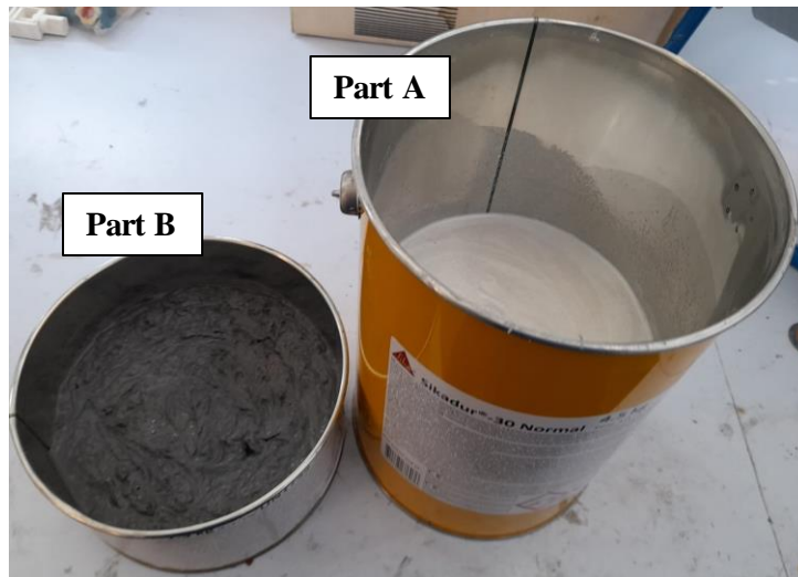
Fig. 3.1 The two-component epoxy adhesive used in this study.
