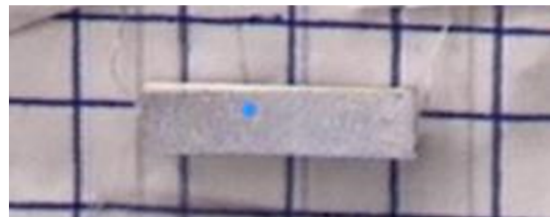
FIGURE 7.3: GaPO_4 PWAS samples used for SLDV measurements (a) PWAS with parallel electrode (b) PWAS with wraparound electrode bonded to Alumina wear plate.
