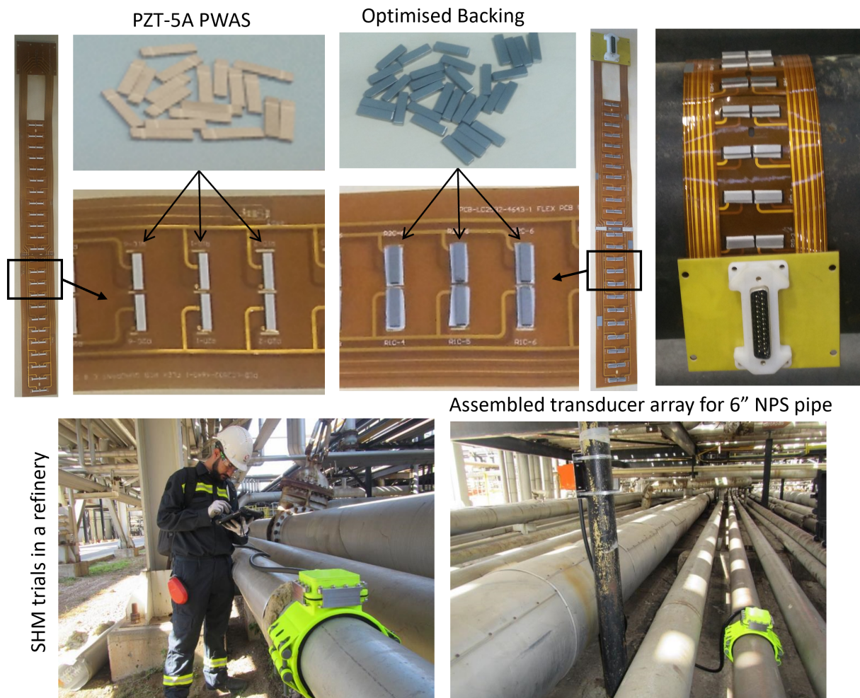
FIGURE 5.19: Design and application of optimised transducer in an array for SHM application in a refinery.
