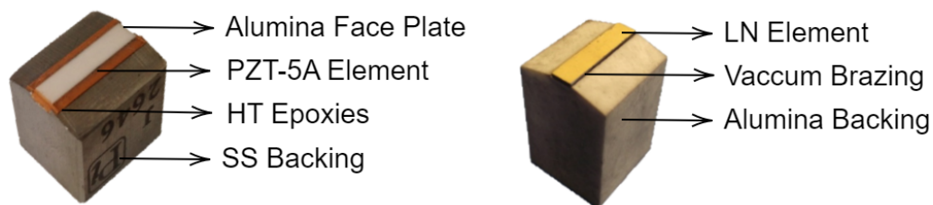
FIGURE 3.2: Previously developed HT-UGW transducers using PZT-5A for operation at 250°C and Lithium Niobate at 580°C [174].
