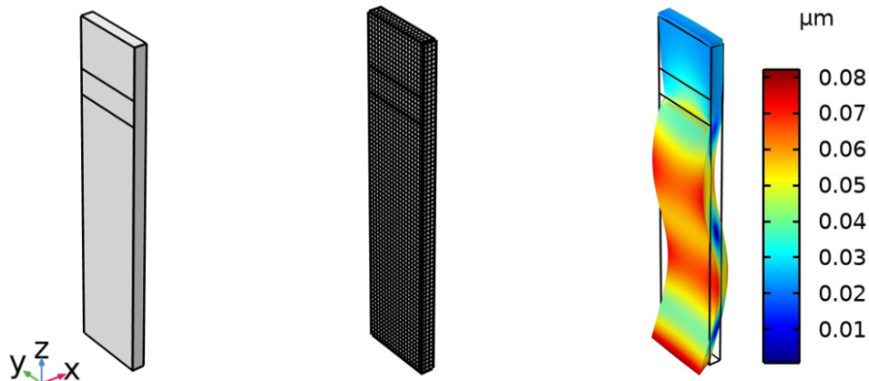
FIGURE 4.2: FEA model geometry, meshing and vibrational response of the PZT-5A piezoelectric wafer transducer.
