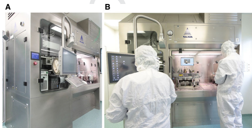
Figure 29. Custom-made GMP-compliant flow cytometric cell sorter (A) with auxiliary equipment cabinet (left) and laminar air flow hood (right) containing the sort chamber and (B) the sort unit in operation (safety-cabinet-enclosed sort unit seen between the two operators).
