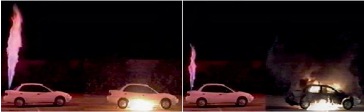
Figure 7. 2: Timeline from 3 seconds to 60 seconds result of having an automotive fire in the Hydrogen and gasoline tank
