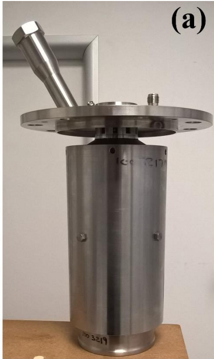
Fig 3 the full size of combustor prototype: (a) swirler, liner and casing, etc (b) fuel injection system
