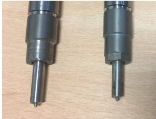
Figure 21: Left - machined injector collar, Right – standard injector collar
