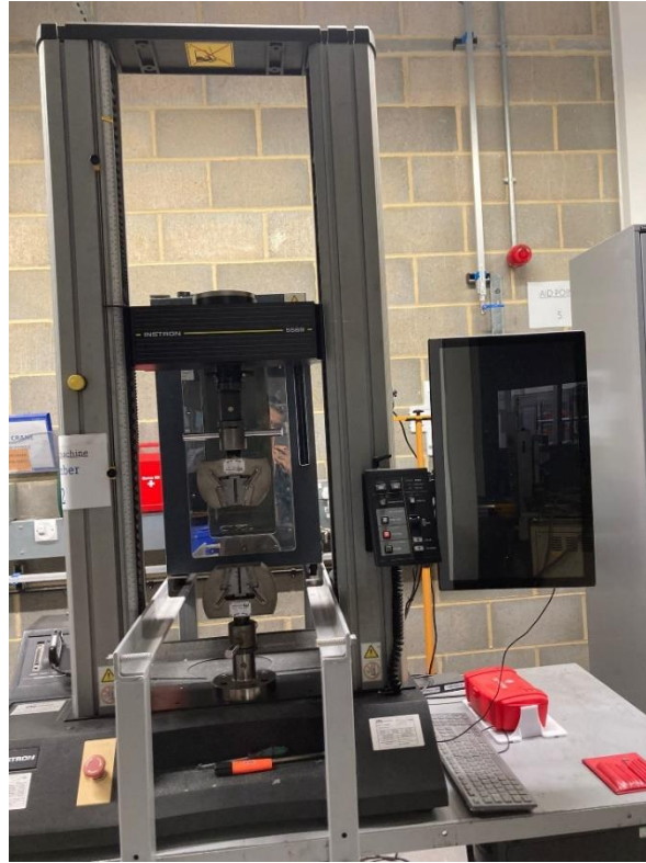
Figure 3.22 Picture of Instron 5500 universal electromechanical tester with ambient and high temperature tensile testing set up.
