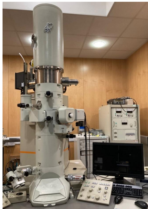
Figure 3.19 The Jeol 2100F Field Emission Gun Transmission Electron Microscope.
