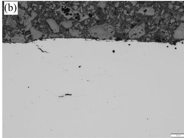
Figure 5.30 Optical Microscope observations of 5mm-thick specimen (a) the whole cross-section (b) the deepest crack
