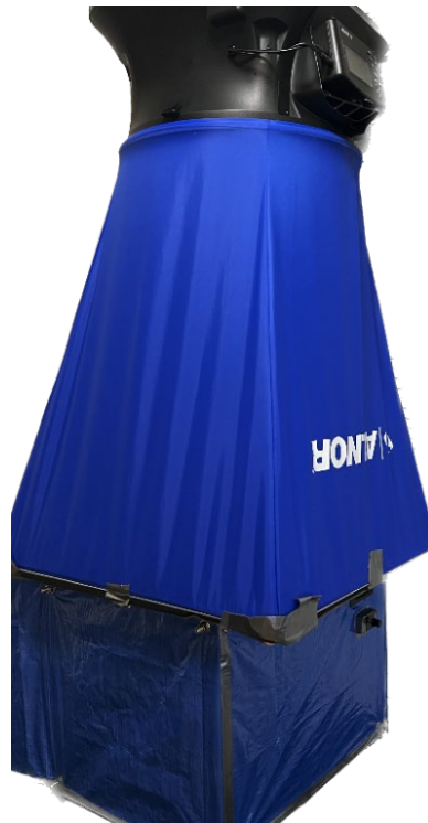
Figure 6-19. Capture Hood Setup Over the SWAC Unit.
