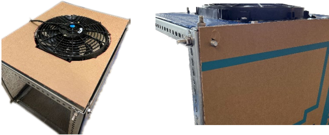
Figure 6-9. Cardboard Panels Covering the Frame Top and Sides.
