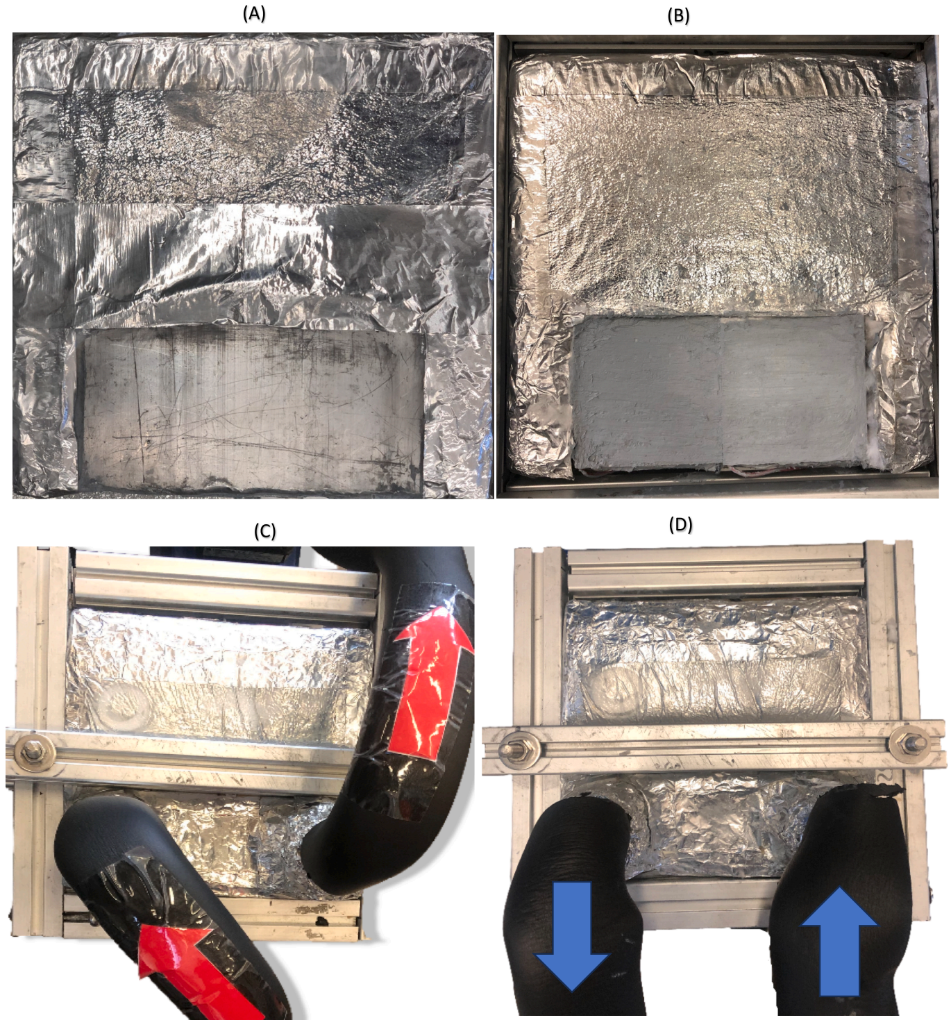
Fig. 4. A) Insulated manifold before placing the TEG. B) Insulated manifold after placing the TEG and the thermal grease C) Top view of the manifold D) Bottom view of the manifold.
