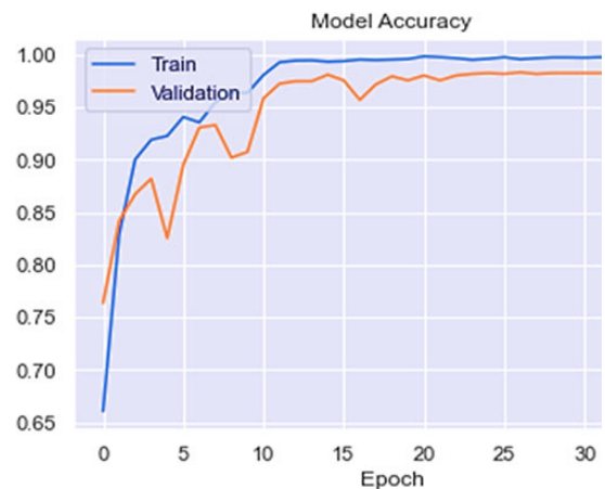
FIGURE 9. Training and validation accuracy trends over 30 Epochs: Demonstrating the convergence and generalisation capabilities of the MoEffNet model.
