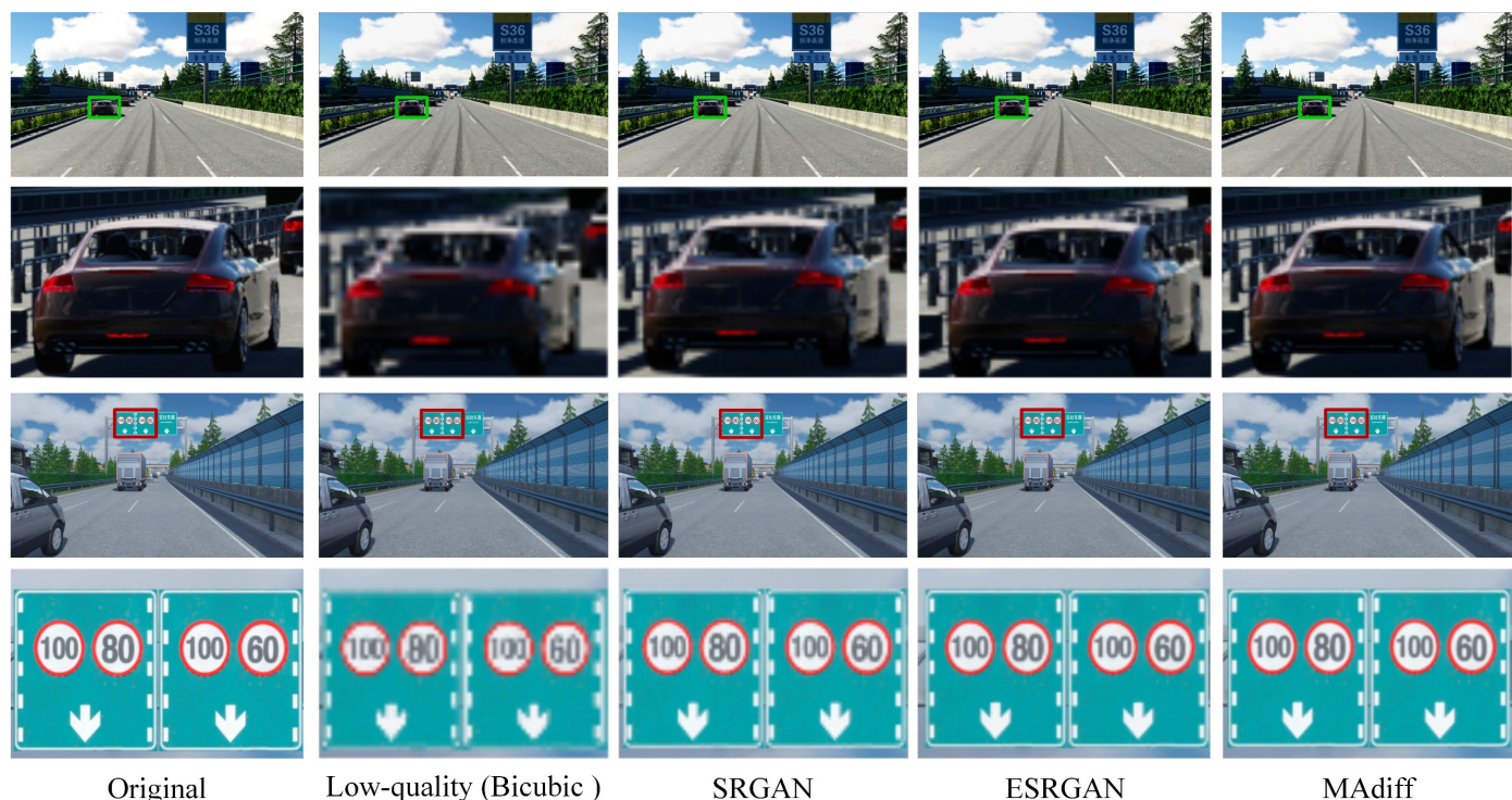
Fig. 7. Super-resolution reconstruction results of different methods on the 51world dataset, where Low-quality represents the result of 4 times bicubic interpolation down-sampling.
