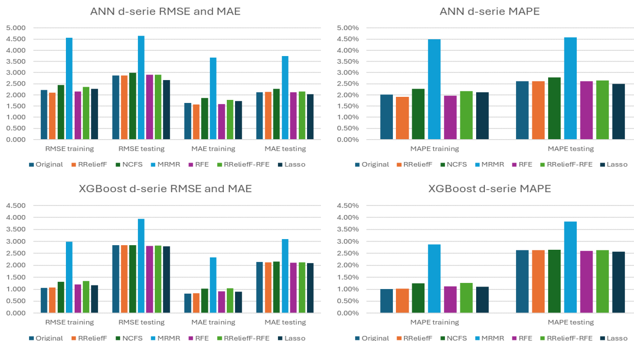
FIGURE 2. Train and Test metrics for all methods for the d-serie module. (Top ANN) (Bottom XGBoost)
