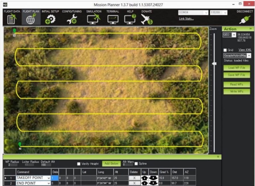
Fig. 4 Regenerative farm monitoring using a mission planner
