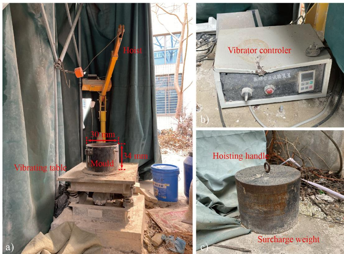
Figure 3.7. Apparatuses for determining the  $\rho_{dmax}$ , including a) a vibrating table, a mould, and a hoist; b) vibrator controller; c) surcharge weight.
