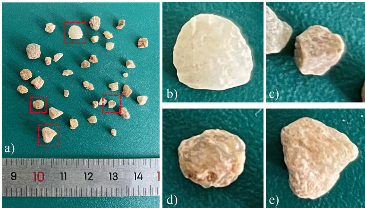
Figure 3.3. River sands with a round particle shape and a smooth surface.
