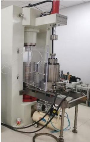
**Fig. 2** QKX-YD-1000 servo-controlled multifunctional rock loading system
