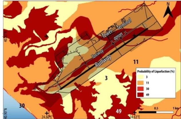
Figure 3. Probability of liquefaction in KVA area.
