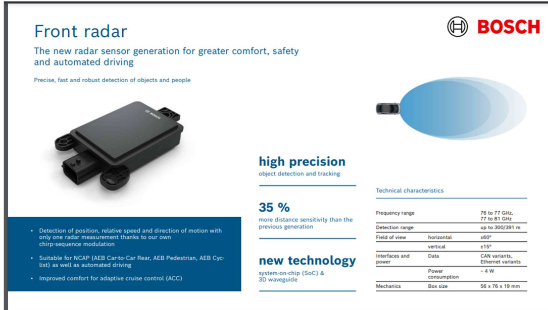
Fig. 6.1: Technical Specification of a Long Range Radar ECU (source: https://www.bosch-mobility.com/ )
