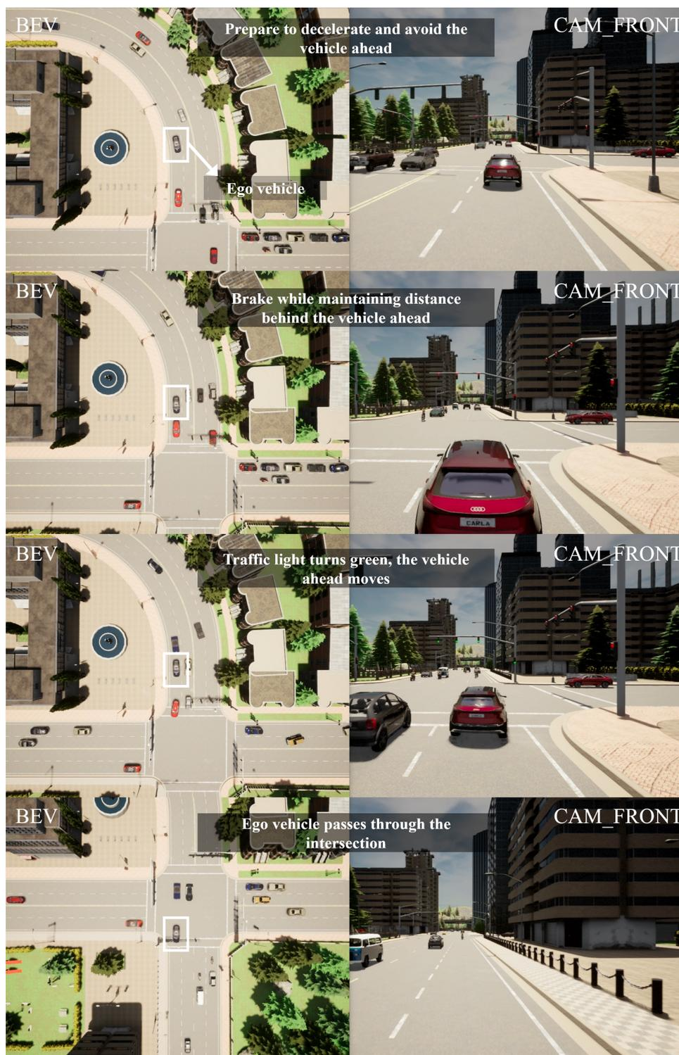
**Figure A1.** Illustration of ego vehicle's decision-making process: waiting for the vehicle ahead and passing through the intersection.
