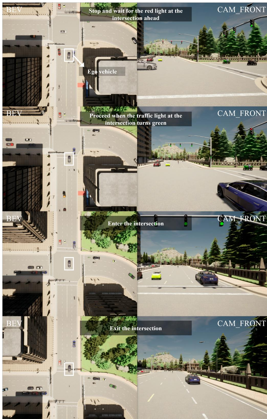
**Figure A2.** Illustration of ego vehicle's decision-making process: waiting and passing through the intersection with a traffic light.
