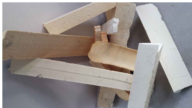
Figure 1. Blocks of rigid polyurethane foams from construction and demolition waste.
