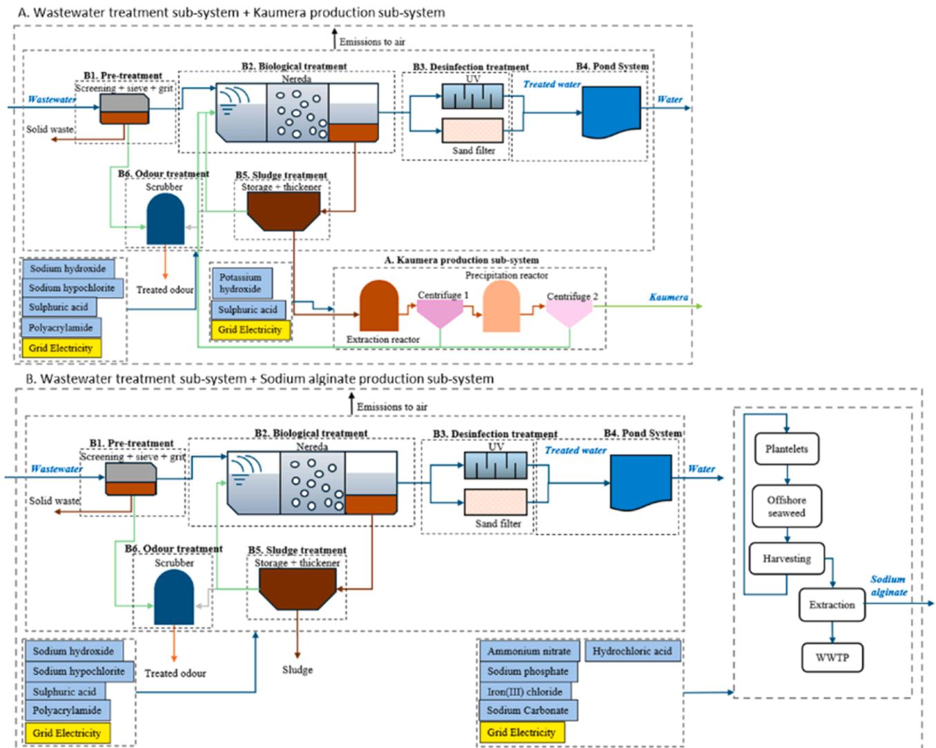
Fig. 1. A: The original system with processes comprising the Kaumera production sub-system and the existing wastewater treatment sub-system; B: The reference system with processes comprising the sodium alginate production sub-system and the existing wastewater treatment sub-system.
