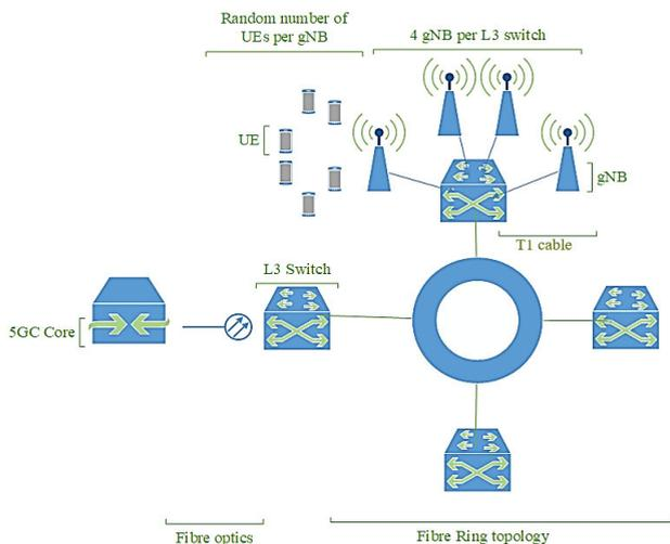
**FIGURE 3.** Fiber optics simulation network layout.
