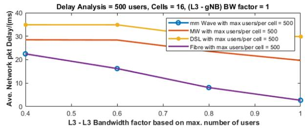
FIGURE 14. Average network packet delay (ms) L3-L3 link.
