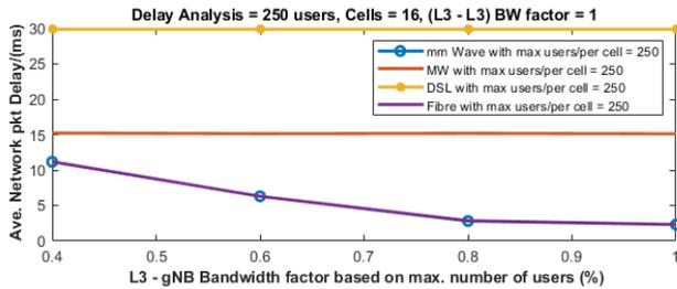
FIGURE 11. Average network packet delay (ms) L3-gNB link.
