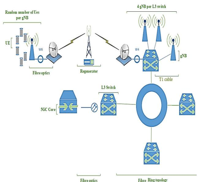
**FIGURE 5.** Microwave simulation network layout.
