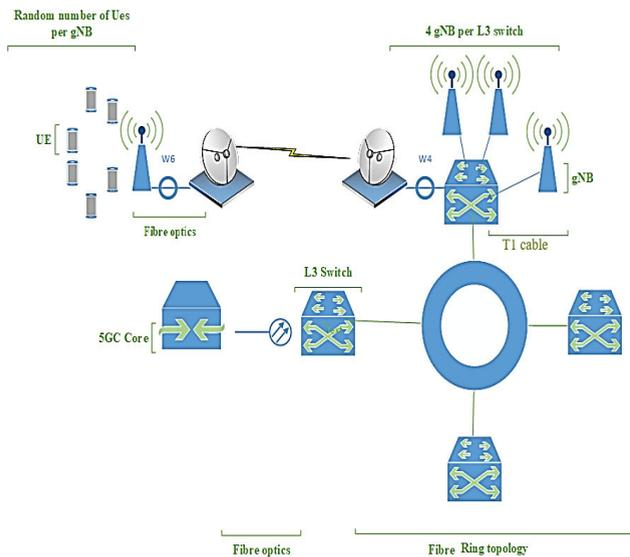
FIGURE 6. mm wave simulation network layout.
