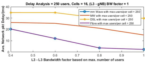
FIGURE 13. Average network packet delay (ms) L3-L3 link.
