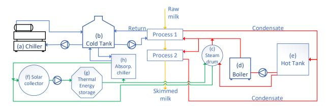
Figure 1: Basic schematic designed for the integration of solar technology in a dairy plant.
