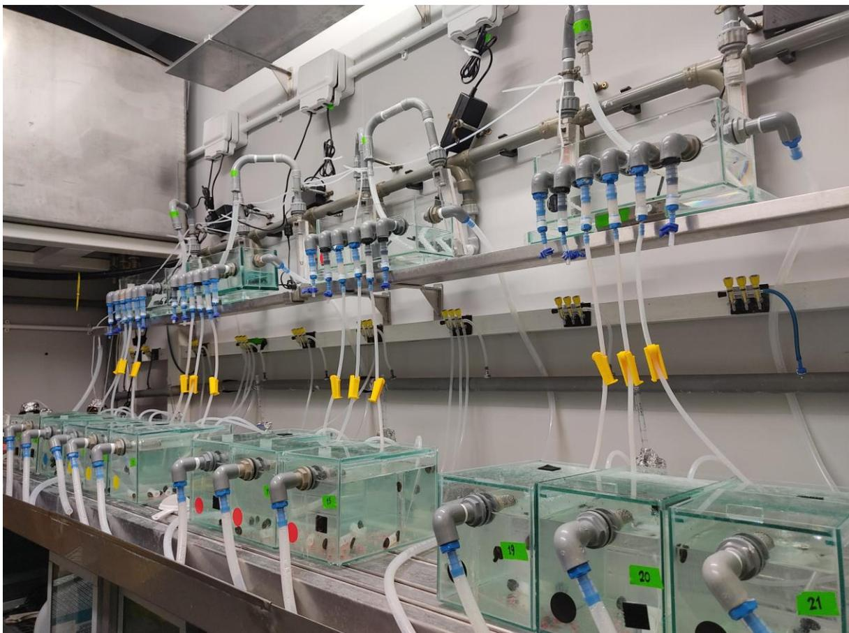
**Figure 4.1:** Flow-through system used for the 21-day reproduction study (Experiment 1). From left to right, pictured are the mixing chambers (above) and replicate tanks (below) for the DWC, 1  $\mu\text{g/L}$ , 10  $\mu\text{g/L}$  and 100  $\mu\text{g/L}$  treatments.
