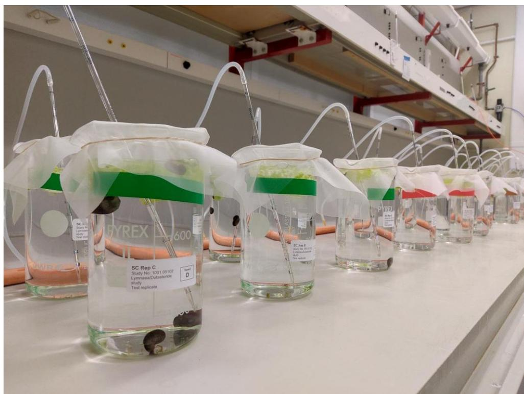
**Figure 4.5:** Static-renewal system used during the 28-day reproduction study. Pictured are the test vessels of SC (green) and 10µg/L (red) treatments.
