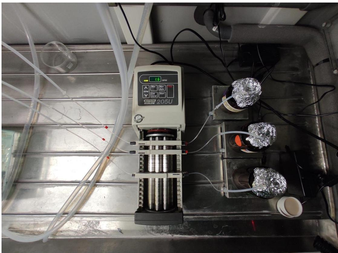
**Figure 4.2:** The finalised dosing stocks of 32 µg/L DUT, 3.2 µg/L DUT and SC from top to bottom, connected to the peristaltic pump via manifold tubing flowing at a rate of 1.6 rpm.
