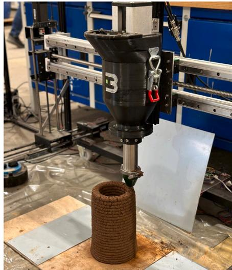
Fig. 3. Extrusion-based 3D printer (Bina Robotics).
