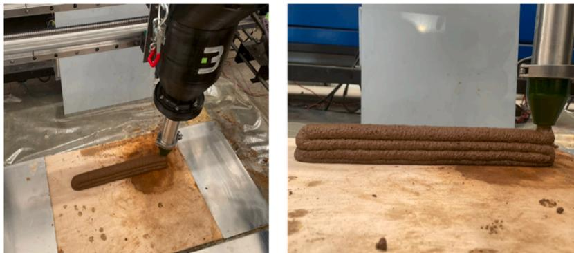
Fig. 4. 3D printed line for extracting prismatic samples for mechanical strength evaluation.
