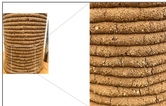
Fig. 13. Layers' printing quality of LC3 with NA (CS mix).
