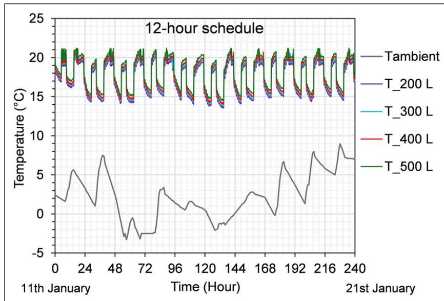
Figure 9. Variation in temperature in the living room for different hot water storage volumes during a 12-hour operating schedule.
