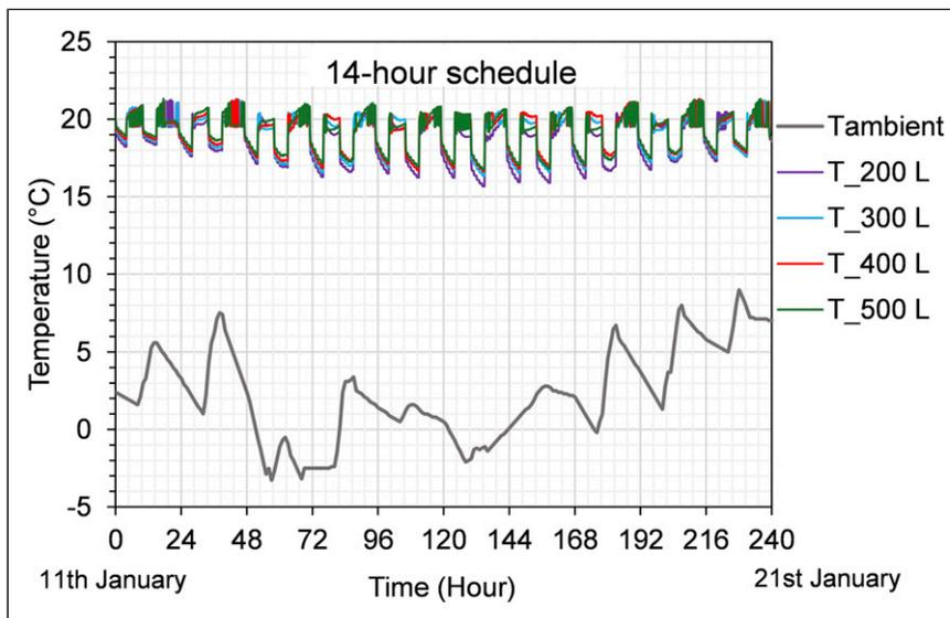
**Figure 12.** Variation in temperature in the living room for different hot water storage volumes during a 14-hour operating schedule.
